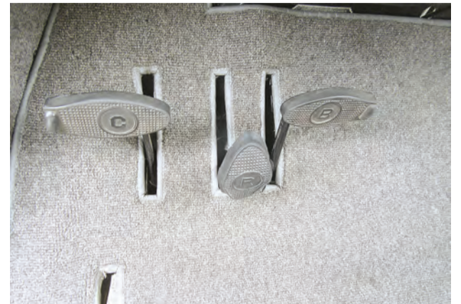
The pedals, left to right, the clutch, reverse and brake.
