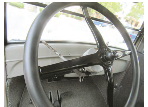
The steering wheel with the spark lever (left) and throttle (right).
